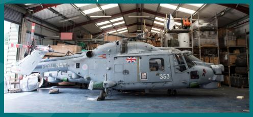
The Lynx HMA8 is a multi-role maritime helicopter with a wheeled undercarriage and deck lock system devised for all-weather operation from Frigate and Destroyer flight decks. It is powered by two Rolls Royce Gem Mk 204 turboshaft engines, each producing 800 SHP (597 kw) at 102.5% Nf. All Up Mass is 5330kgs.
